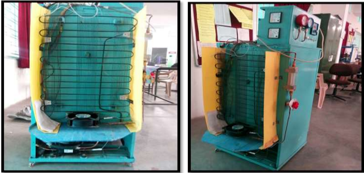
Fig 1 : Fabrication of refrigerator unit with measuring devices.
